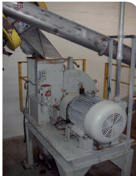
Hammer mills are used to process raw material into a uniform size
